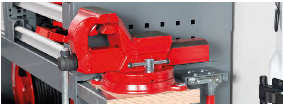
The workbench always travels along, it takes up hardly any room in the vehicle itself, and at the place of use it can be pulled out as required with a few quick hand movements and secured with the quick action retainer.
